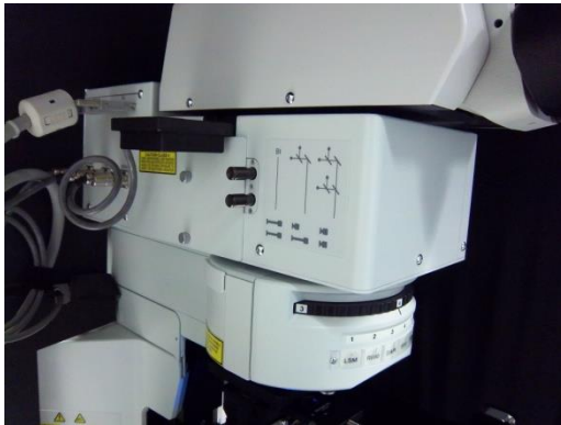
Light to detectors, SDM570 engaged RXD1 (CFP), RXD2 (YFP), and RXD4 (RFP) available.
